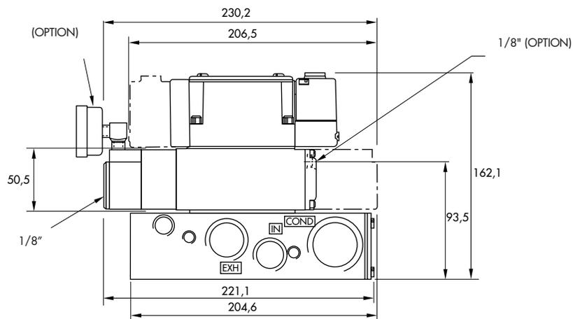
**Sandwich pressure regulator with manual adjust knob.**
