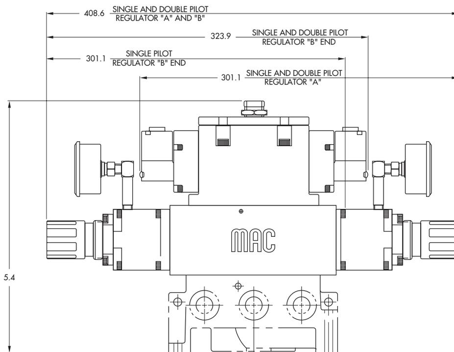
**Sandwich pressure regulator with air pilot adjust.**
