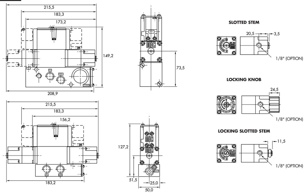
**Sandwich pressure regulator with air pilot adjust.**
