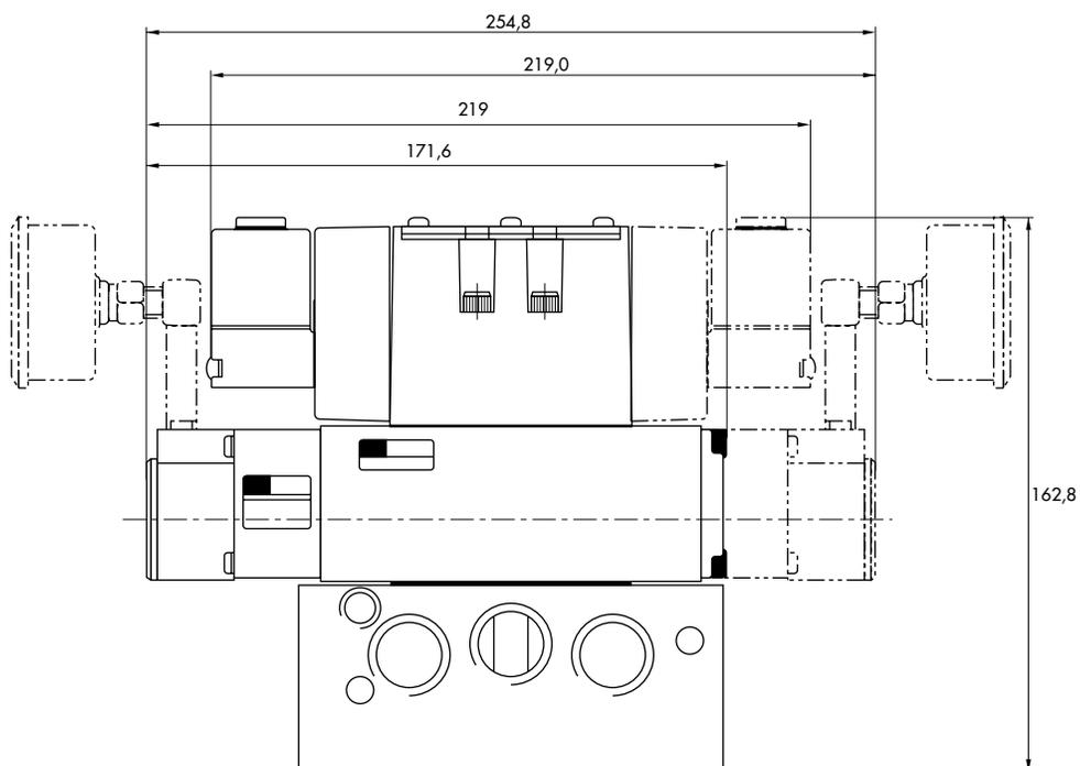
**Sandwich pressure regulator with manual adjust knob.**
