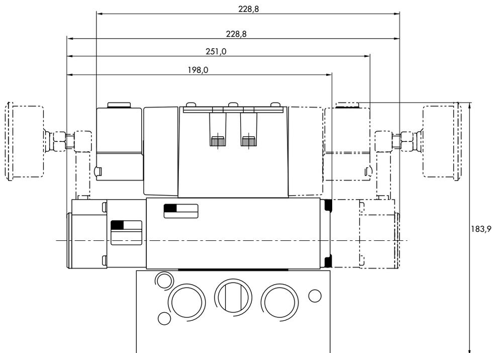
**Sandwich pressure regulator with manual adjust knob.**
