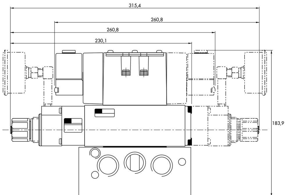
**Sandwich pressure regulator with air pilot adjust.**
