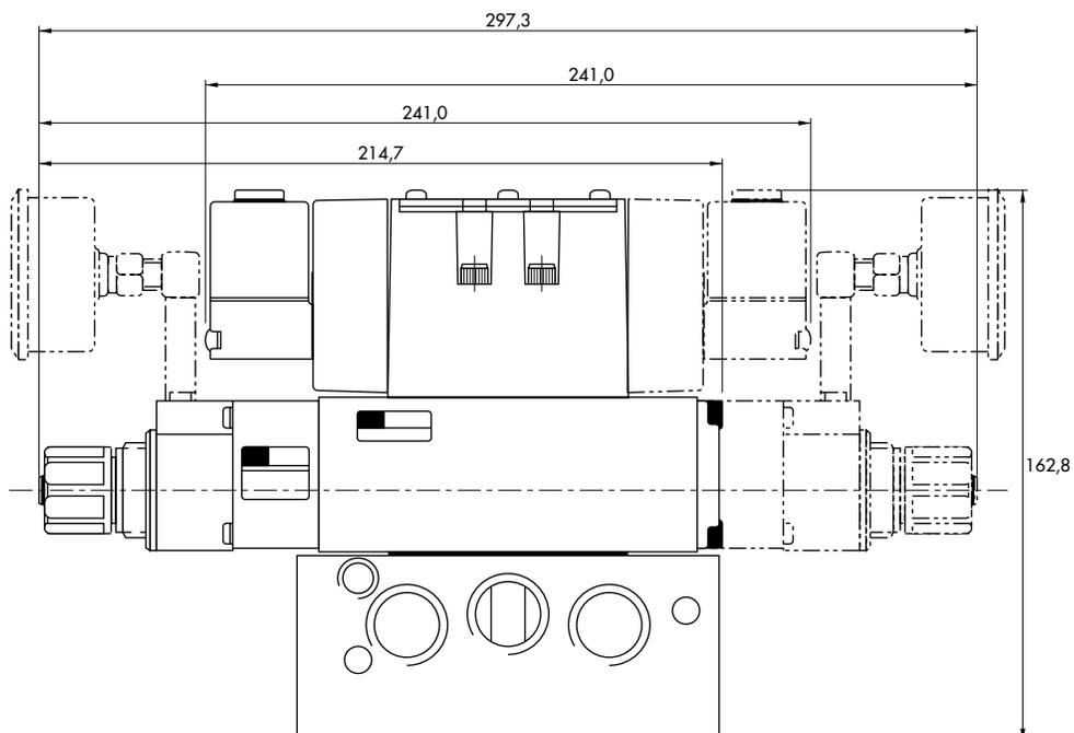
**Sandwich pressure regulator with air pilot adjust.**
