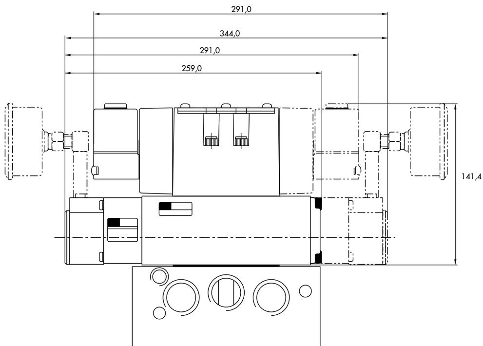
**Sandwich pressure regulator with manual adjust knob.**
