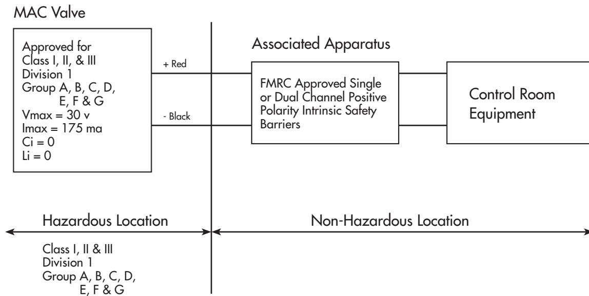
There are 3 basic parts to an intrinsically safe circuit :
