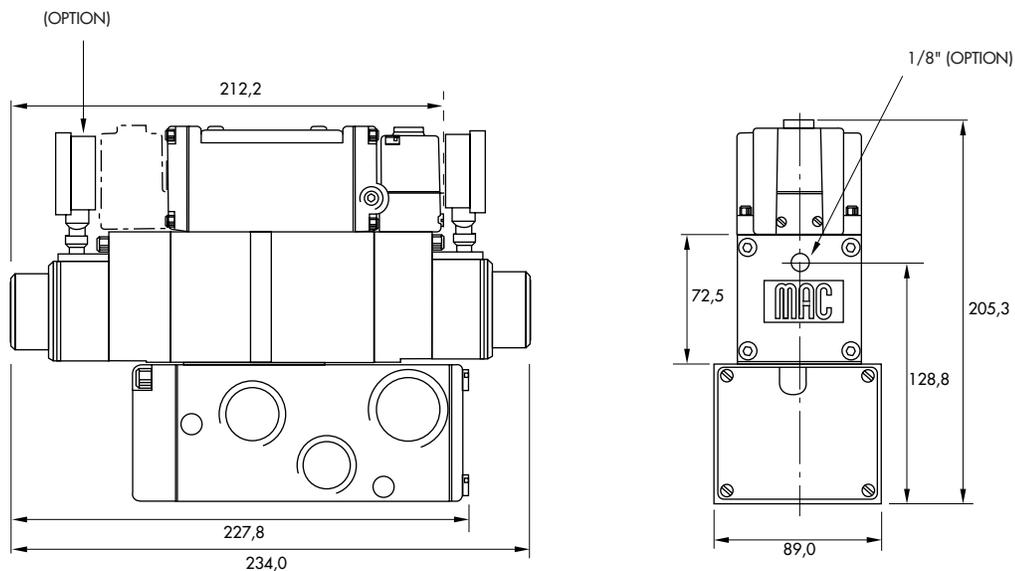
**Sandwich pressure regulator with manual adjust knob.**
