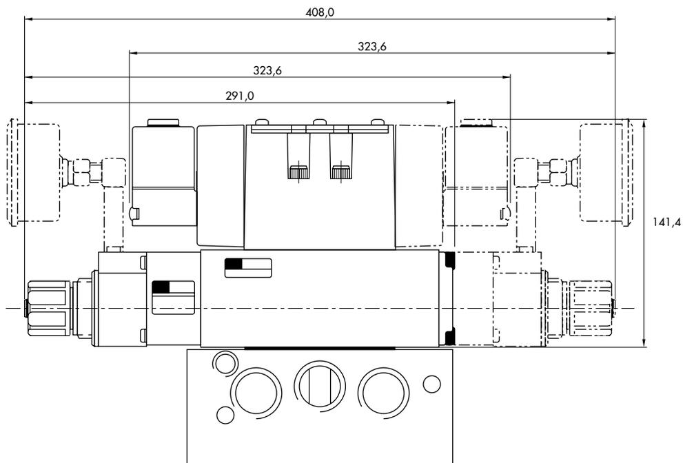
**Sandwich pressure regulator with air pilot adjust.**
