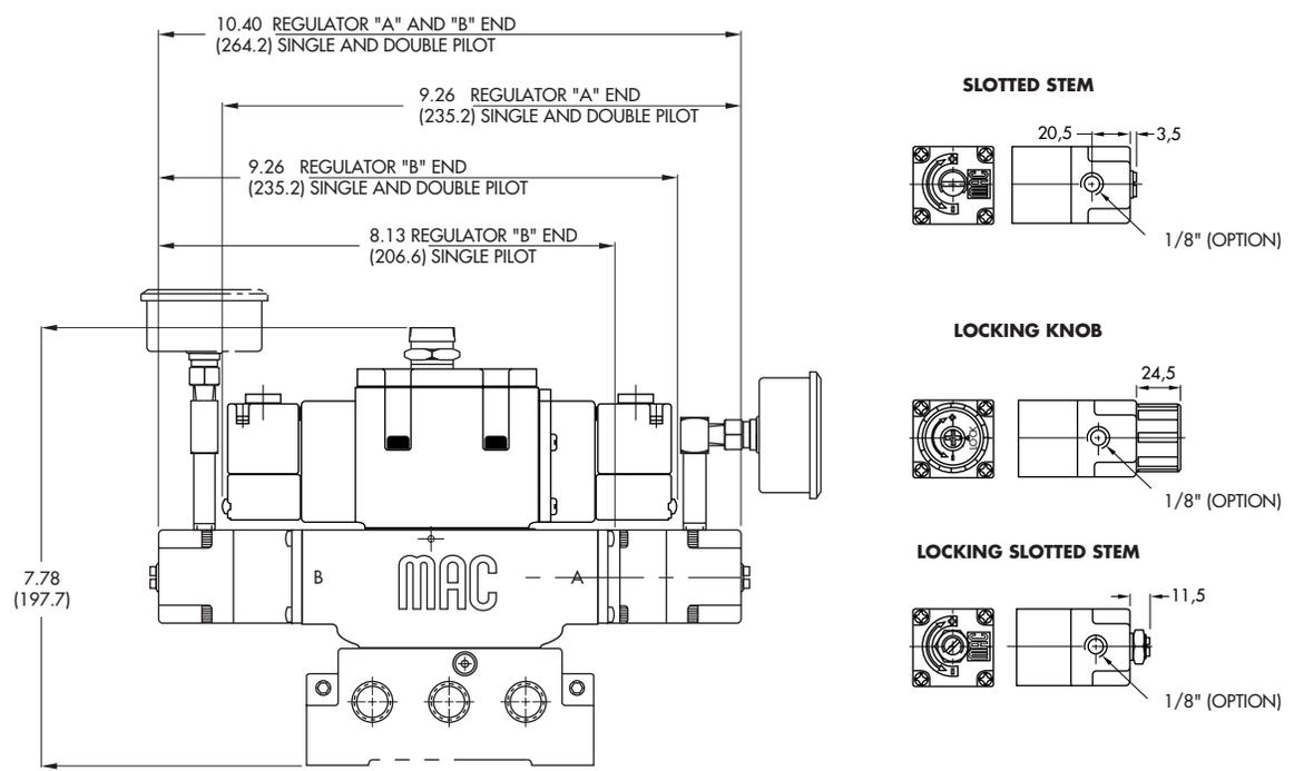
**Sandwich pressure regulator with air pilot adjust.**
