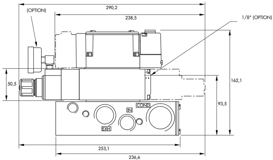
**Sandwich pressure regulator with air pilot adjust.**
