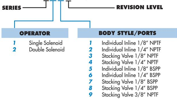
For stacking valve 3/8"BSPP ports, use MOD 0005 after complete valve code 919B-FM-A51BA MOD 0005.
