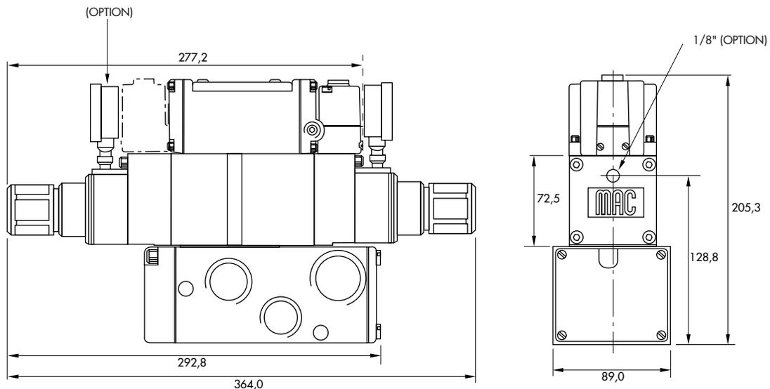
**Sandwich pressure regulator with air pilot adjust.**
