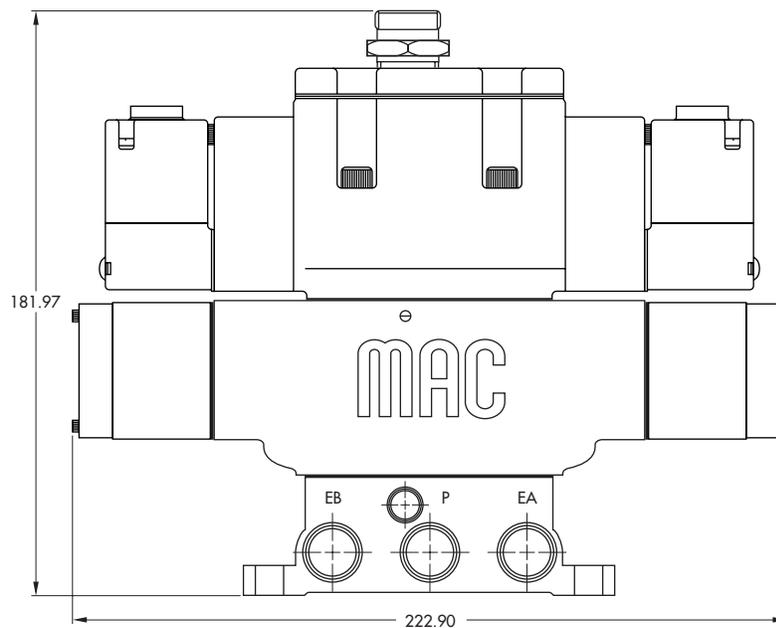
**Sandwich pressure regulator with manual adjust knob.**
